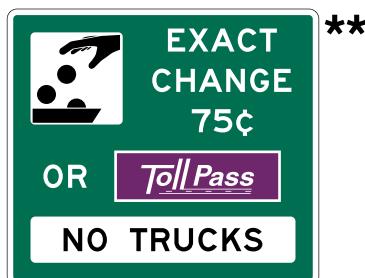
Exact Change or ETC Account lane with an M4-18 Exact Change symbol
