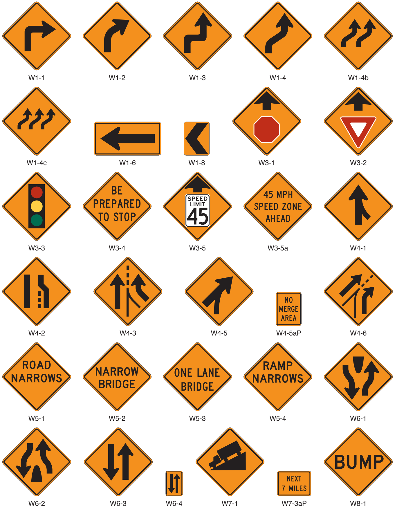
Figure 6H-1. Warning Signs and Plaques in Temporary Traffic Control Zones (Sheet 1 of 4)
