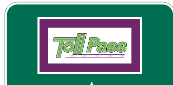
2. Pictograph with a purple underlay on a non-contrasting background
