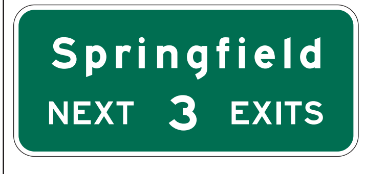
Figure 2E-33. NEXT EXITS Sign
