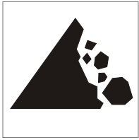
RG-070 FALLING ROCK
