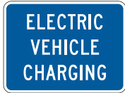
D9-11bP Electric Vehicle Charging
