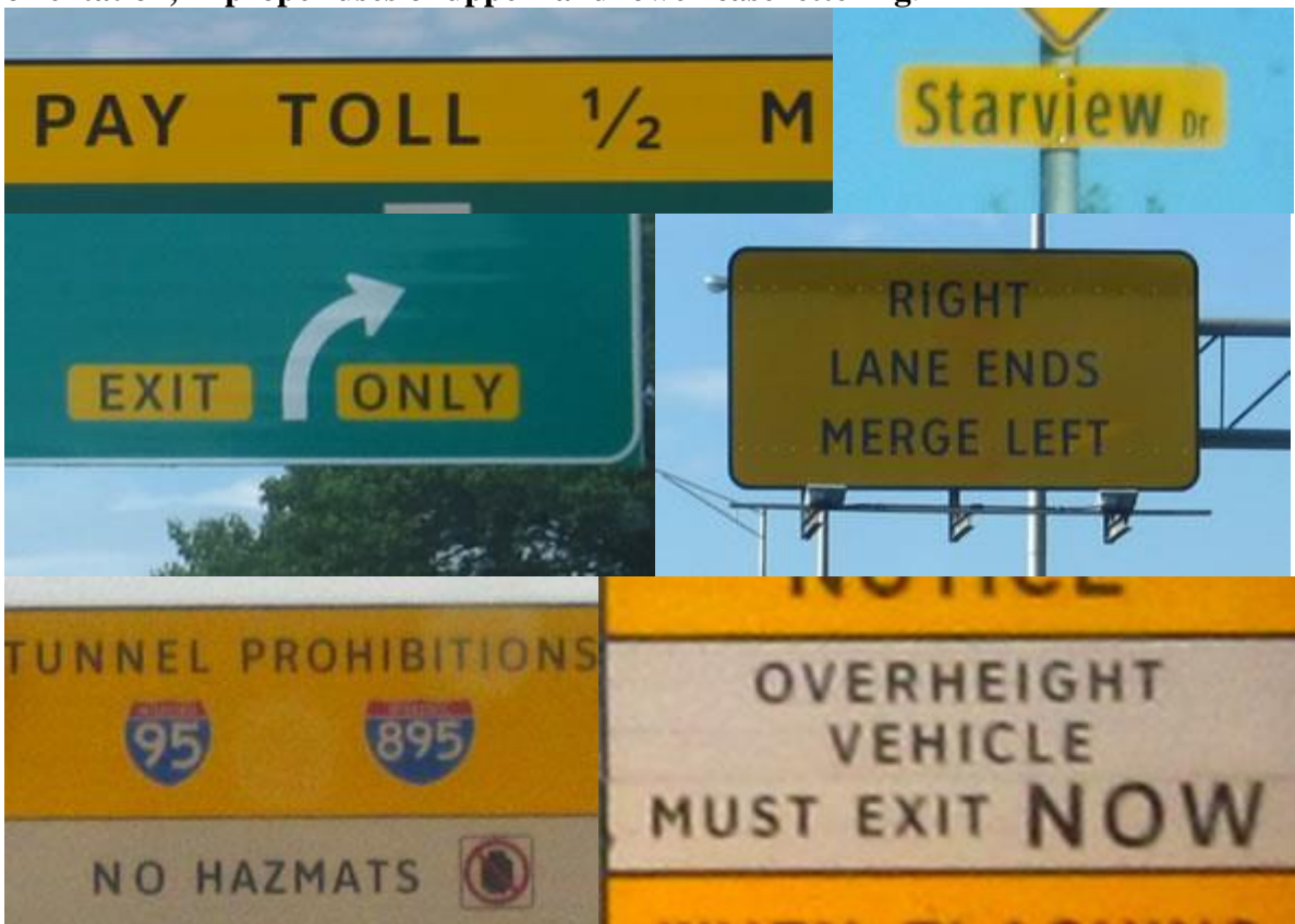
Figure 1b. NOT ACCEPTABLE: Improper uses of Clearview in negative-contrast orientation.
