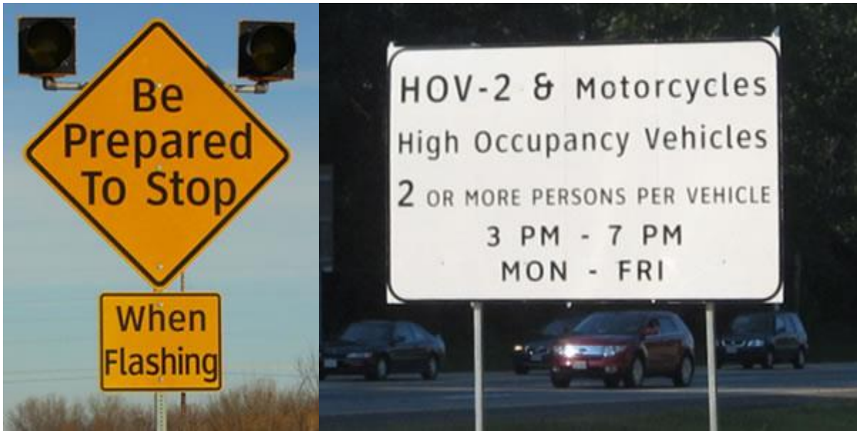
Figure 1a. NOT ACCEPTABLE: Improper uses of Clearview in negative-contrast orientation, improper uses of upper- and lower-case lettering.
