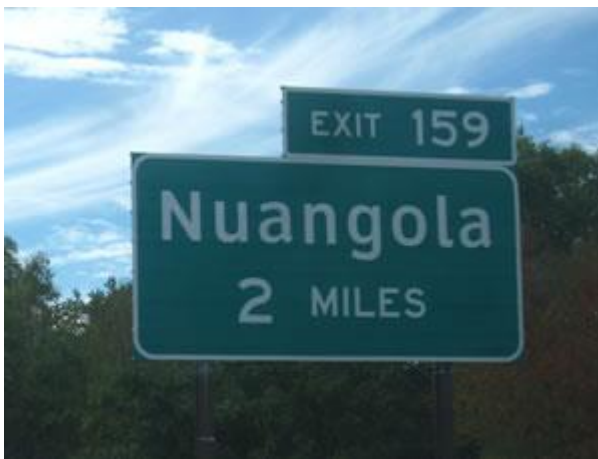
Figure 4. ACCEPTABLE: Example of appropriate use of Clearview for destination legend (mixed-case) and FHWA Standard Alphabets for other legends (all upper-case and numerals).
