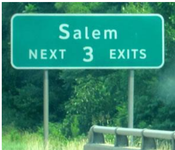
Figure 3. NOT ACCEPTABLE: Incorrect proportion of lower-case loop height (undersized) to initial upper-case letter height.
