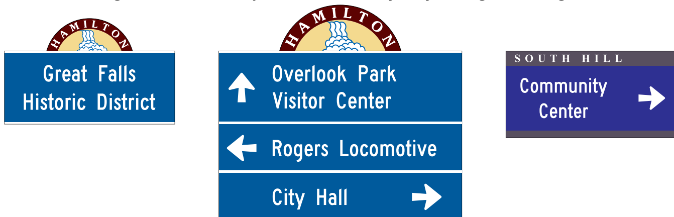
Figure 2D-30. Examples of Community Wayfinding Guide Signs
