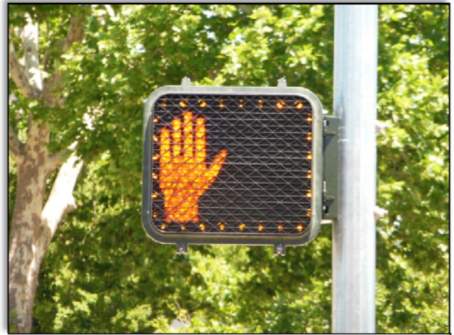
Pedestrian push button is activated (LED border - illuminated)
