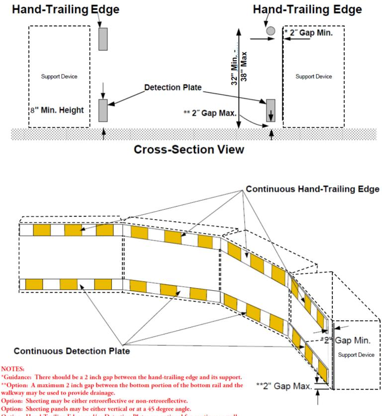
Option: Hand-Trailing Edges and/or Detection Plates are optional for continuous walls.
