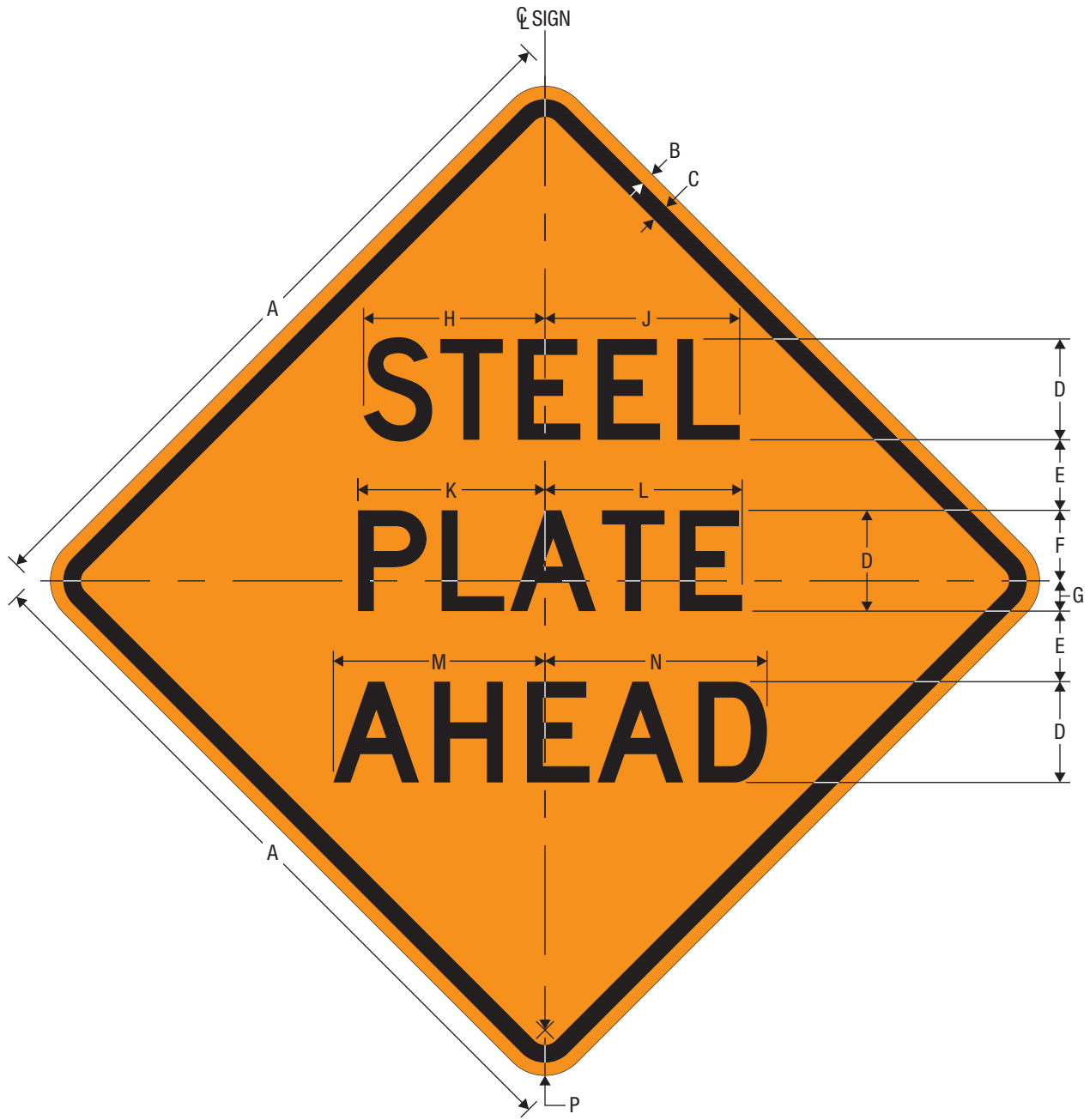
W8-24 STEEL PLATE AHEAD
