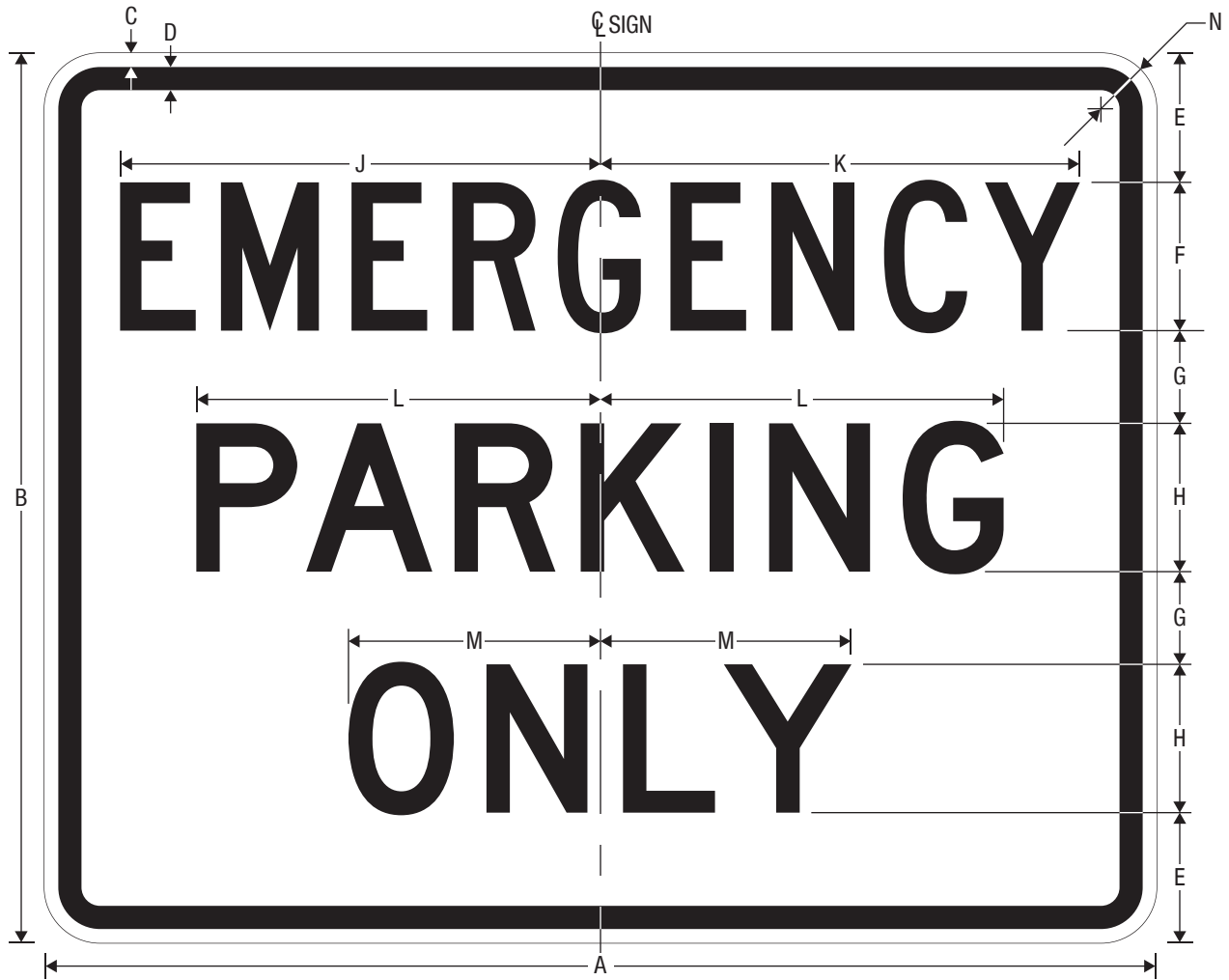
R8-4 EMERGENCY PARKING ONLY
