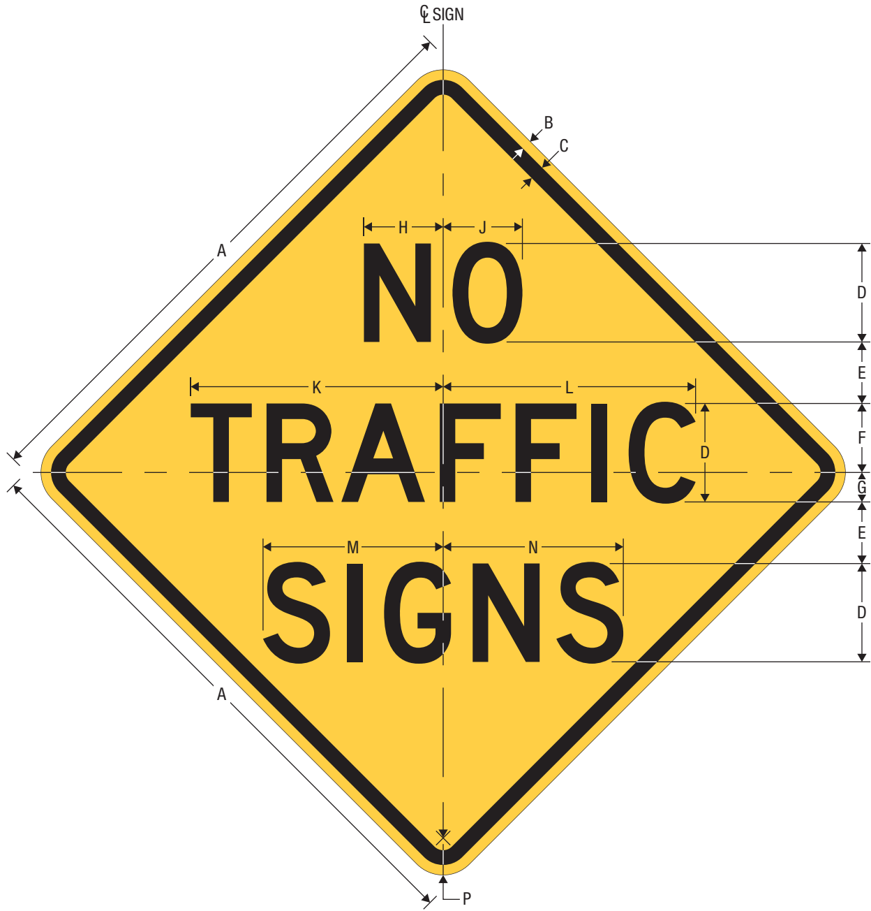
W18-1 NO TRAFFIC SIGNS
