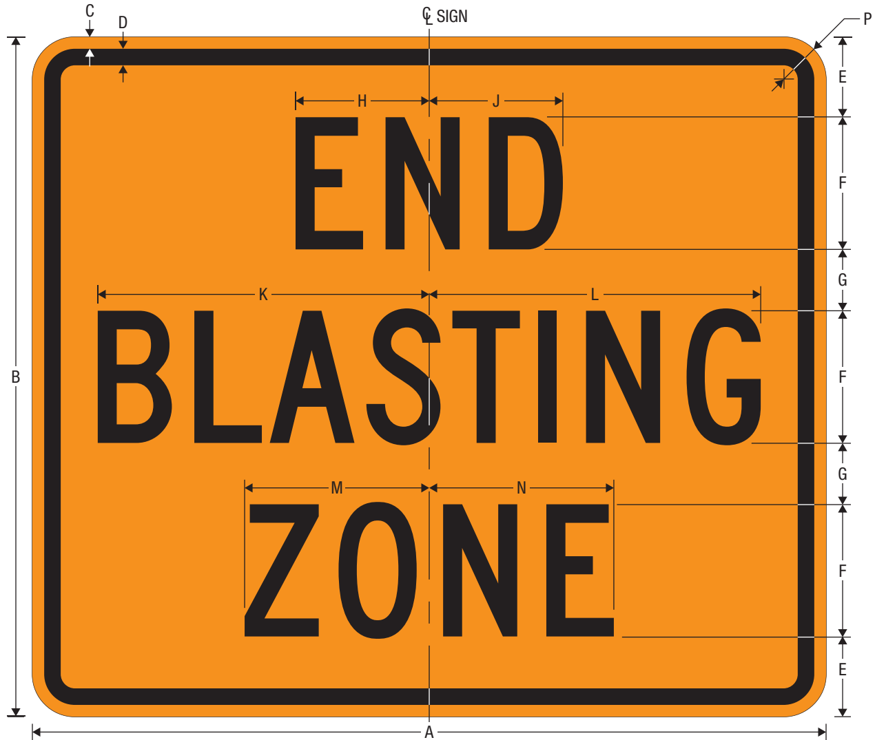
W22-3 END BLASTING ZONE
