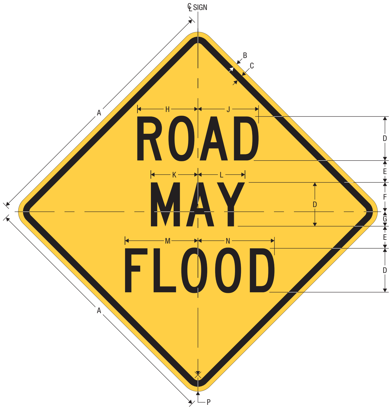
W8-18 ROAD MAY FLOOD
