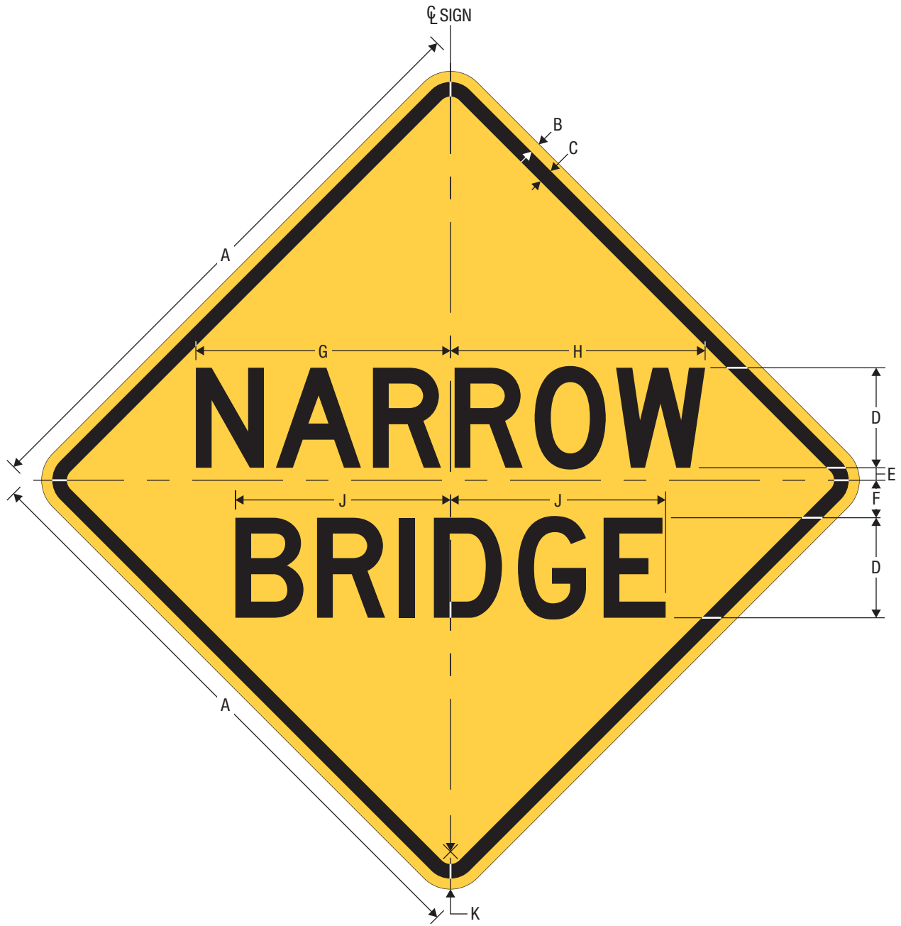
W5-2 NARROW BRIDGE
