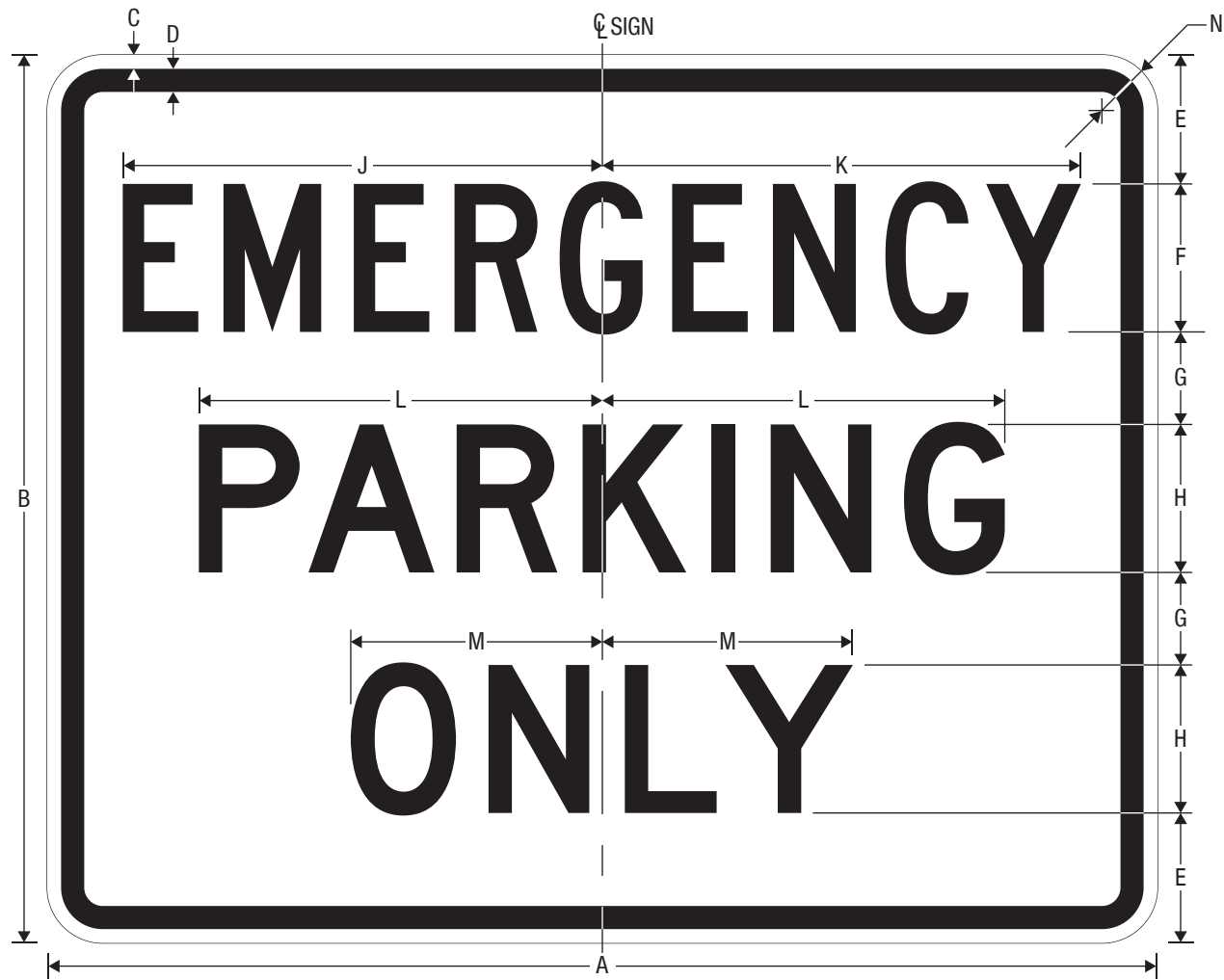
R8-4 EMERGENCY PARKING ONLY
