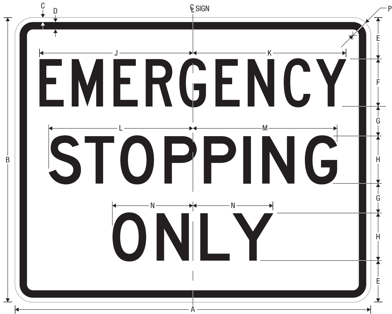
R8-7 EMERGENCY STOPPING ONLY
