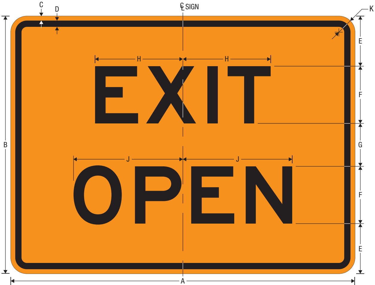
E5-2 EXIT OPEN
