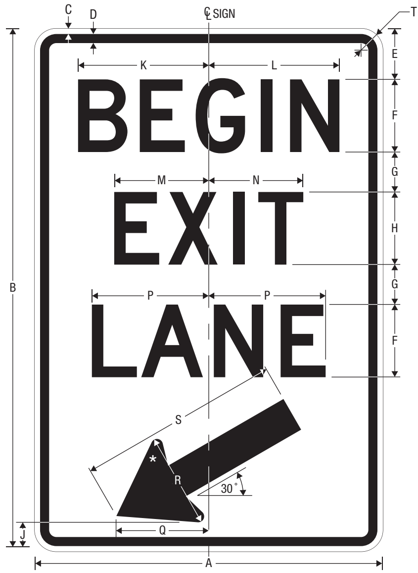
R3-56R BEGIN EXIT LANE
