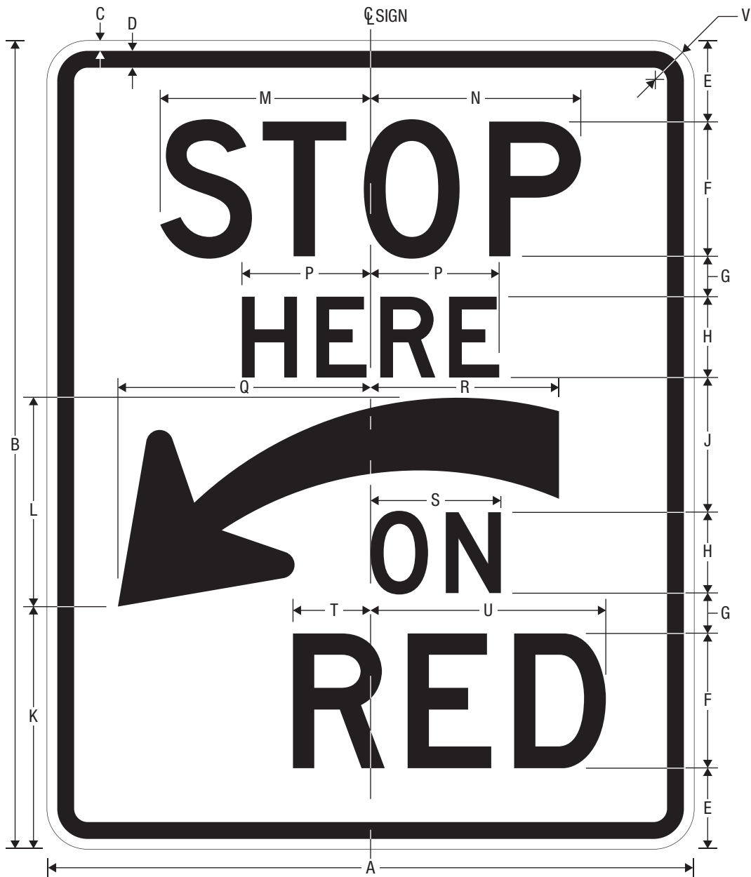
R10-6aL STOP HERE ON RED
