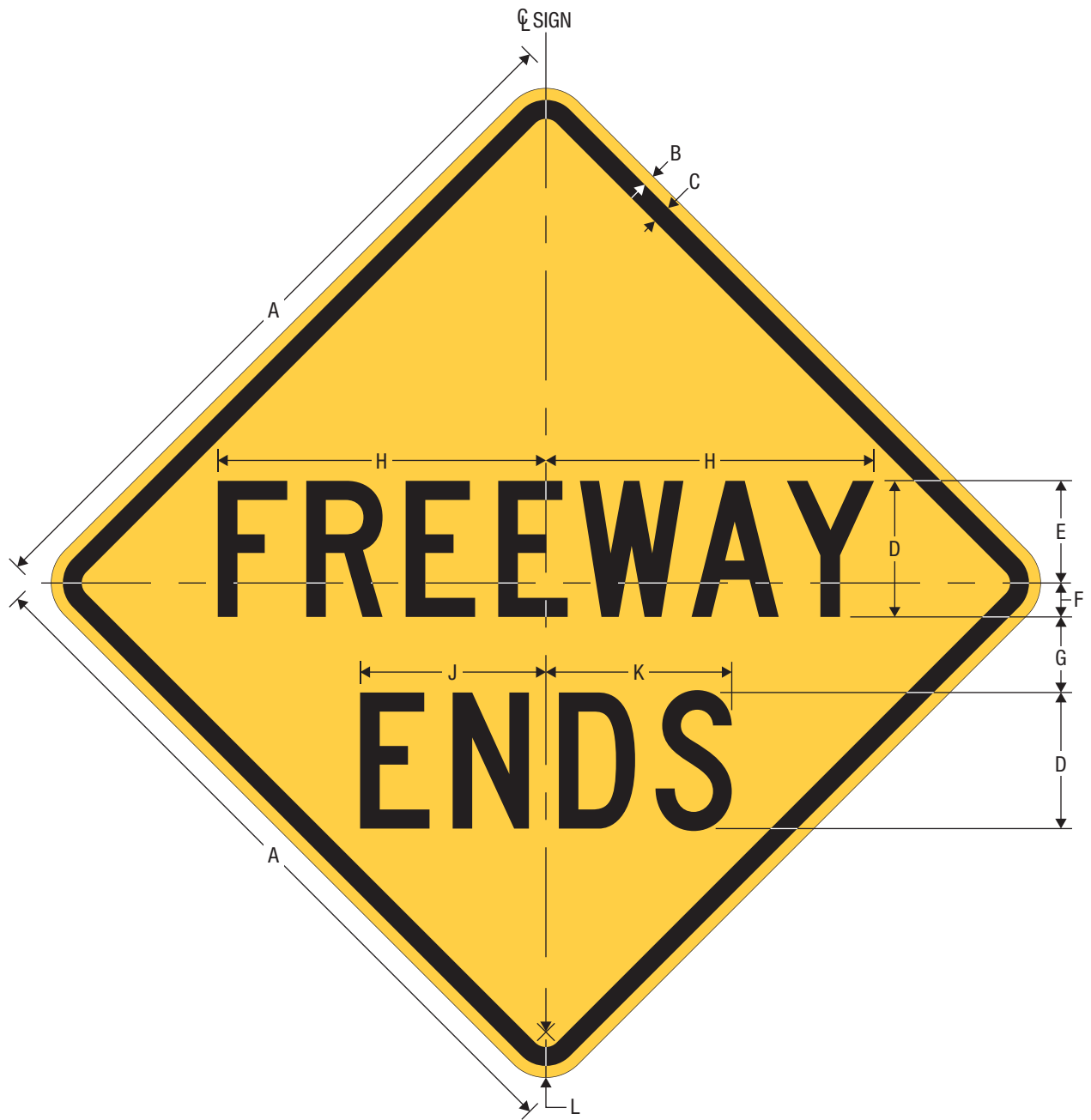
W19-3 FREEWAY ENDS
