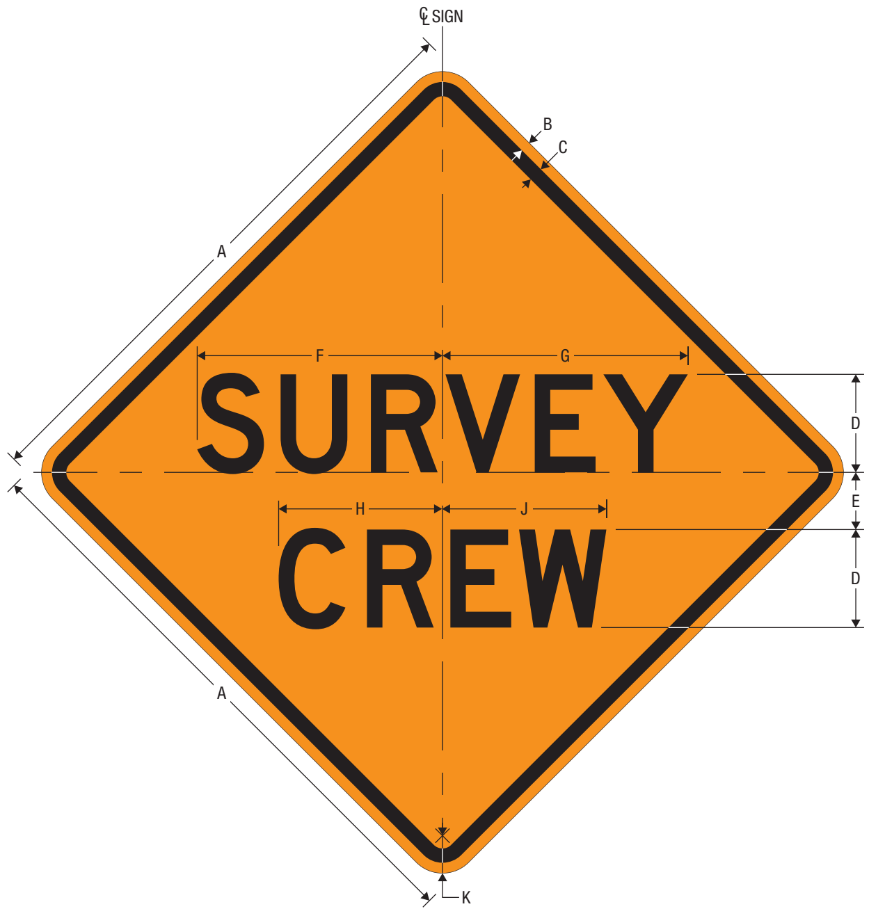
W21-6 SURVEY CREW
