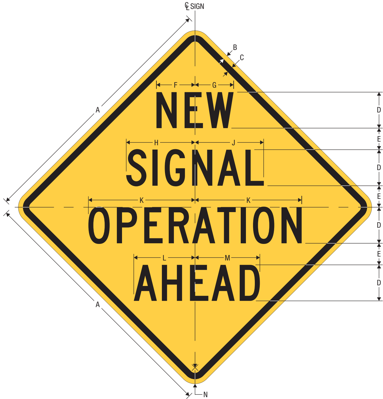
W23-2a NEW SIGNAL OPERATION AHEAD
