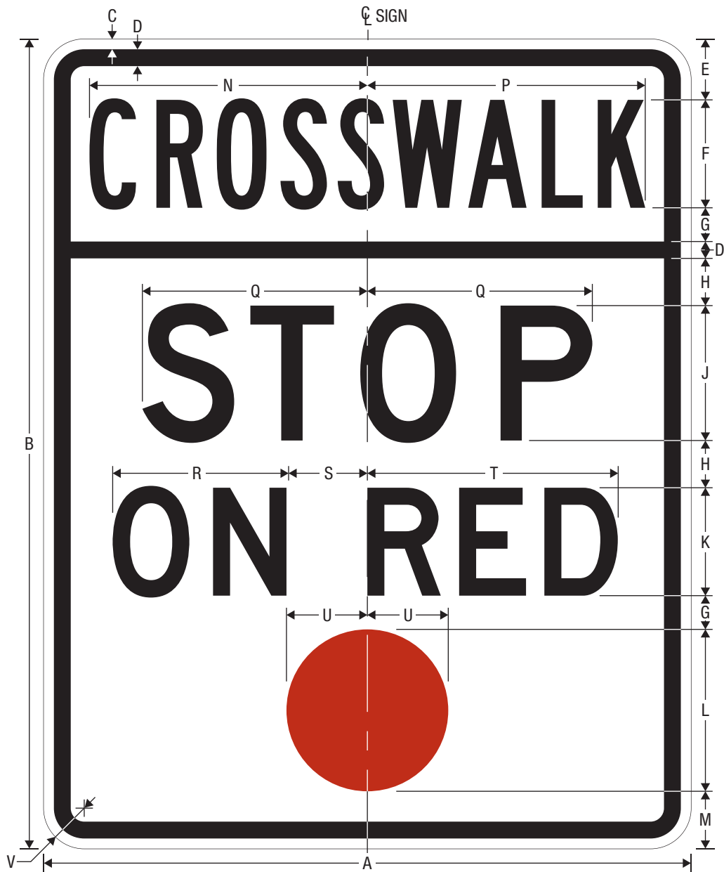
R10-23 CROSSWALK - STOP ON RED
