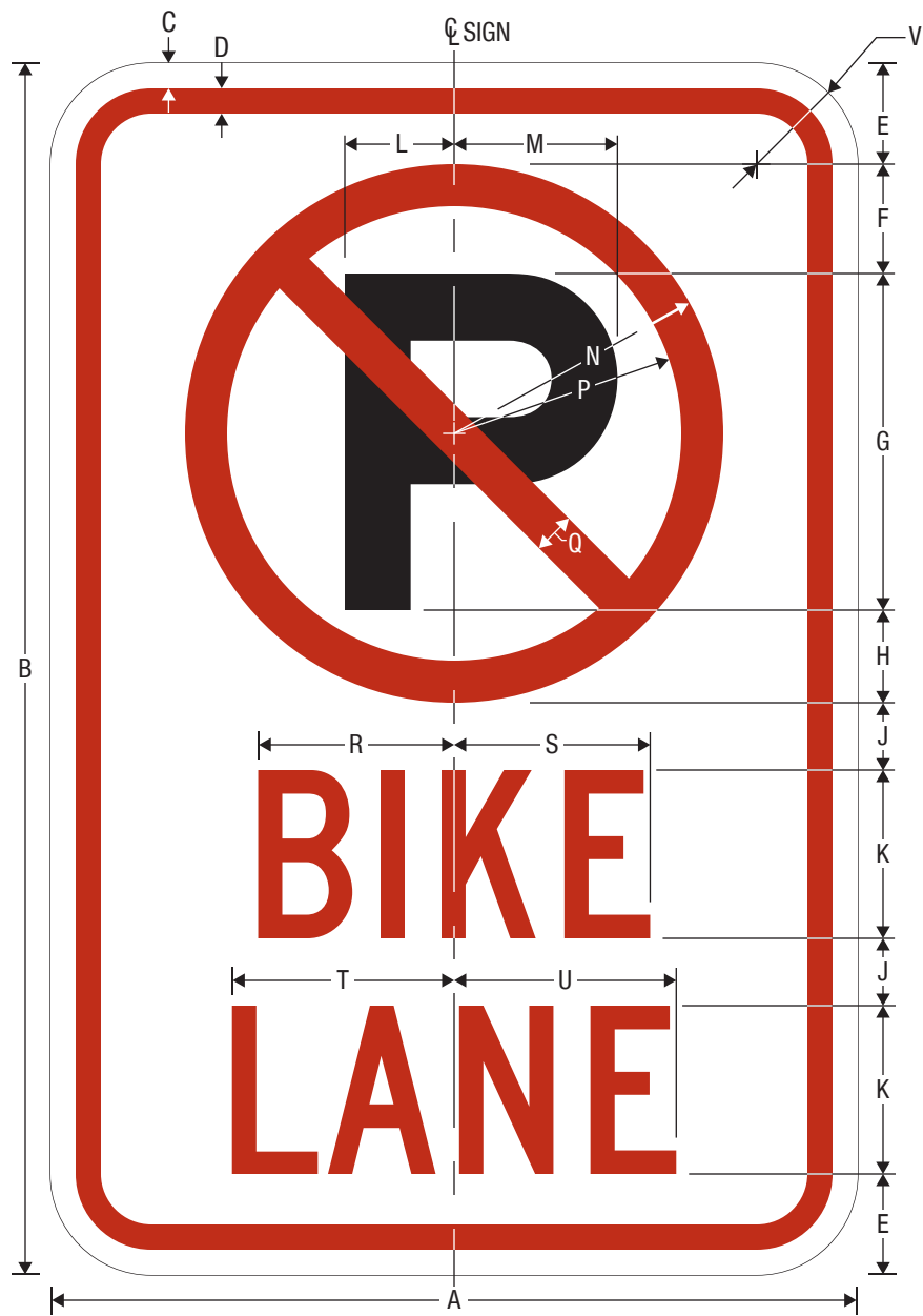
R7-9a NO PARKING BIKE LANE
