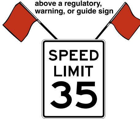
Figure 2A-1. Examples of Enhanced Conspicuity for Signs
