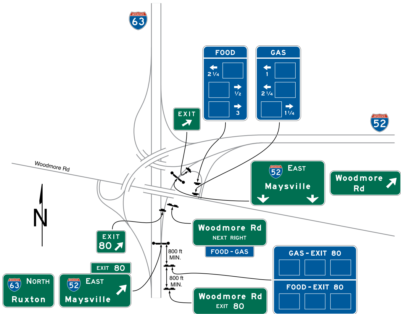
Figure 2J-5. Example of Specific Services Signing for a Conventional Road Accessed within a Freeway-to-Freeway Interchange
