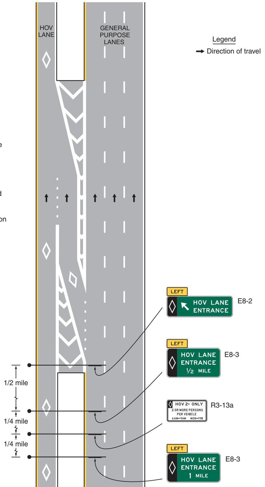
**Figure 2G-10. Example of Signing for the Intermediate Entry to, Egress from, and End of Access-Restricted HOV Lanes**
