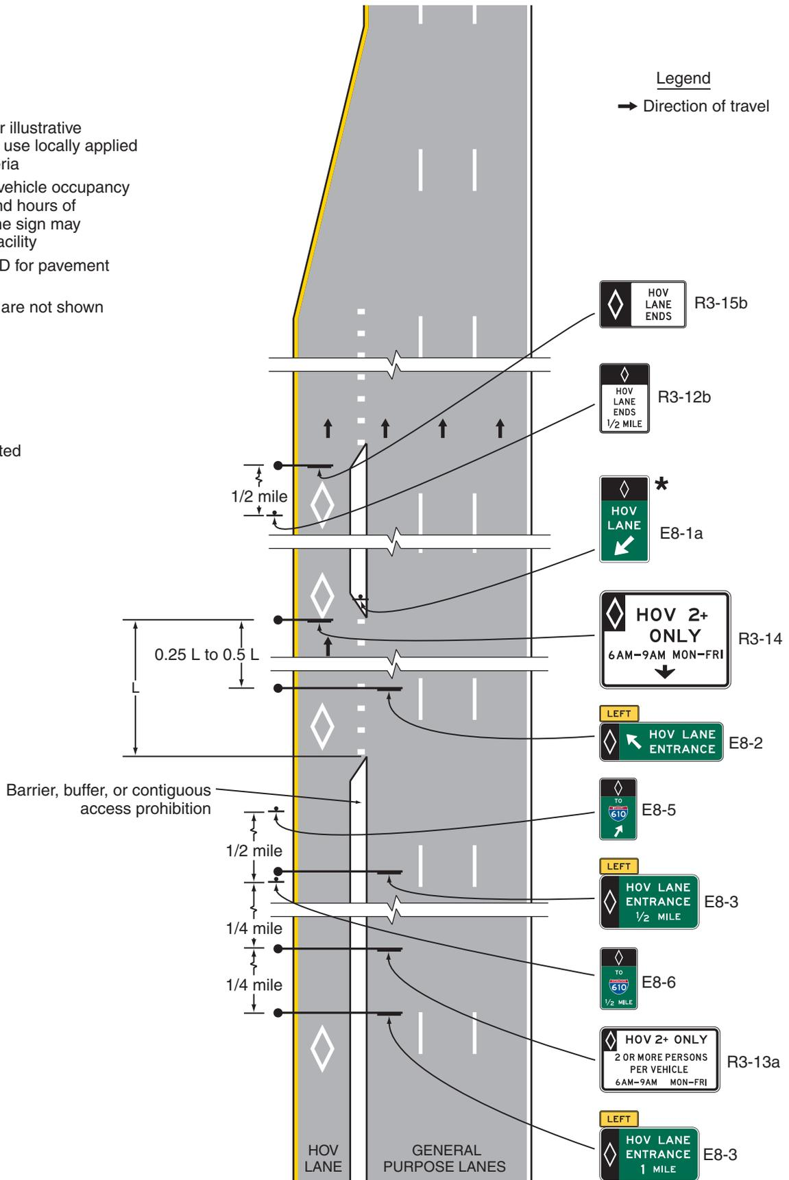
**Figure 2G-11. Examples of Barrier-Mounted Guide Signs for an Intermediate Egress from Preferential Lanes**
