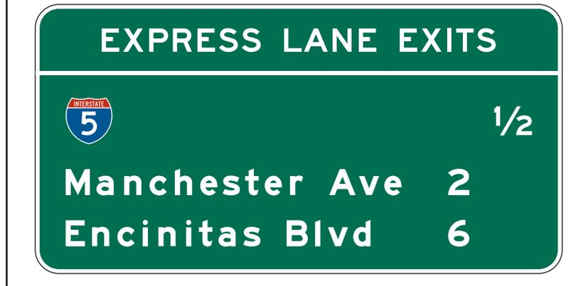
**Figure 2G-20. Example of a Comparative Travel Time Information Sign for Preferential or Managed Lanes**
