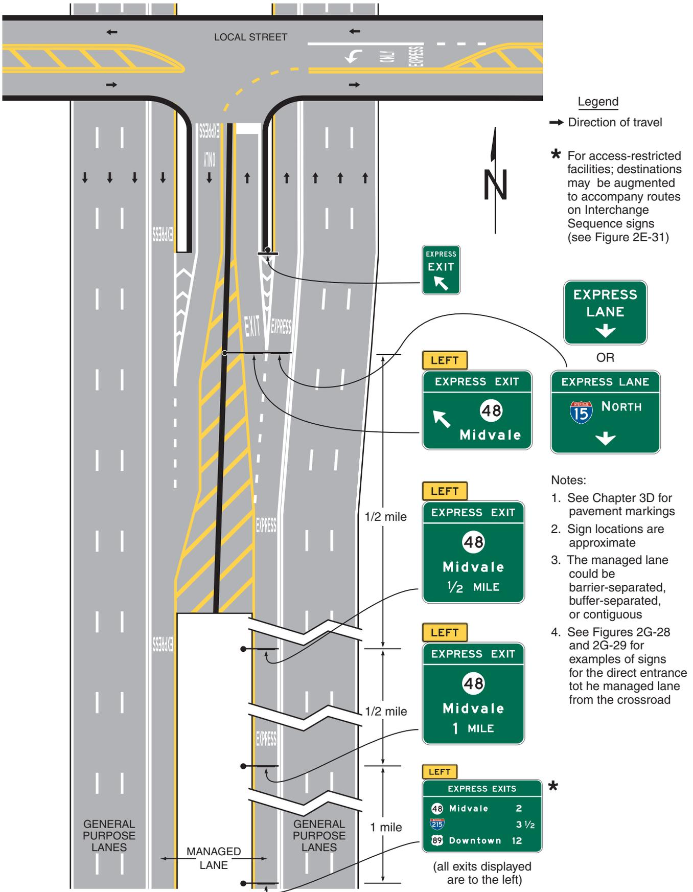
**Figure 2G-27. Examples of Guide Signs for a Direct Access Ramp between Managed Lanes on Separate Freeways**
