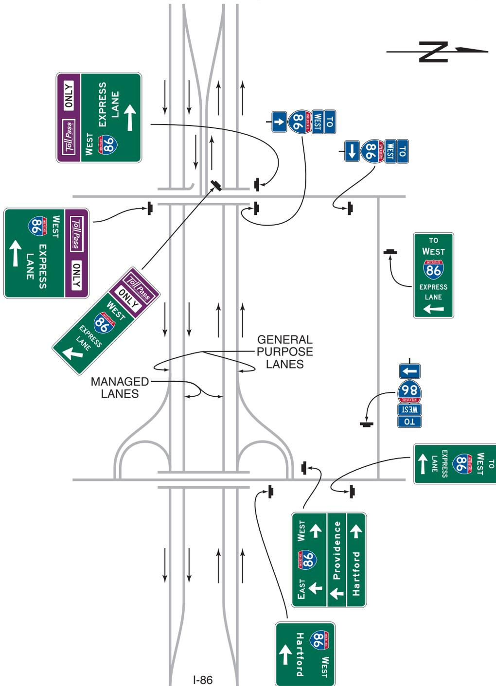
**Figure 2G-29. Examples of Guide Signs for Separate Entrance Ramps to General-Purpose and Priced Managed Lanes from the Same Crossroad**
