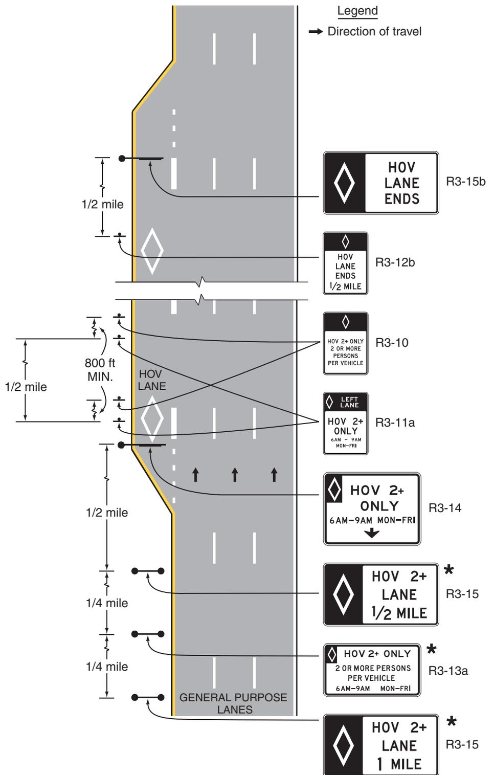
**Figure 2G-3. Example of Signing for a General-Purpose Lane that Becomes a Continuous-Access Contiguous or Buffer-Separated HOV Lane**
