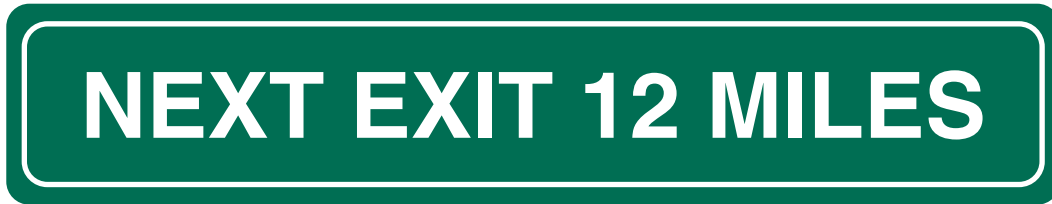
Figure 2E-16. Next Exit Supplemental Advance Guide Signs
