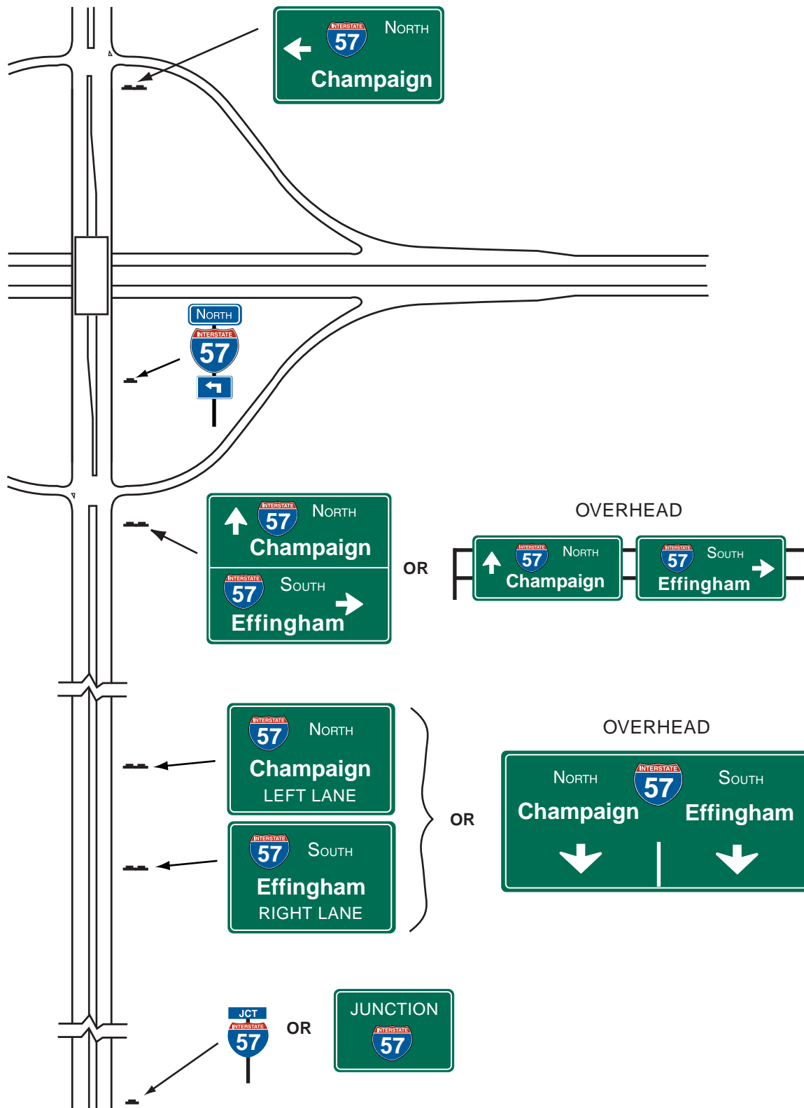
Figure 2E-35. Examples of Multilane Crossroad Signing for Diamond Interchange
