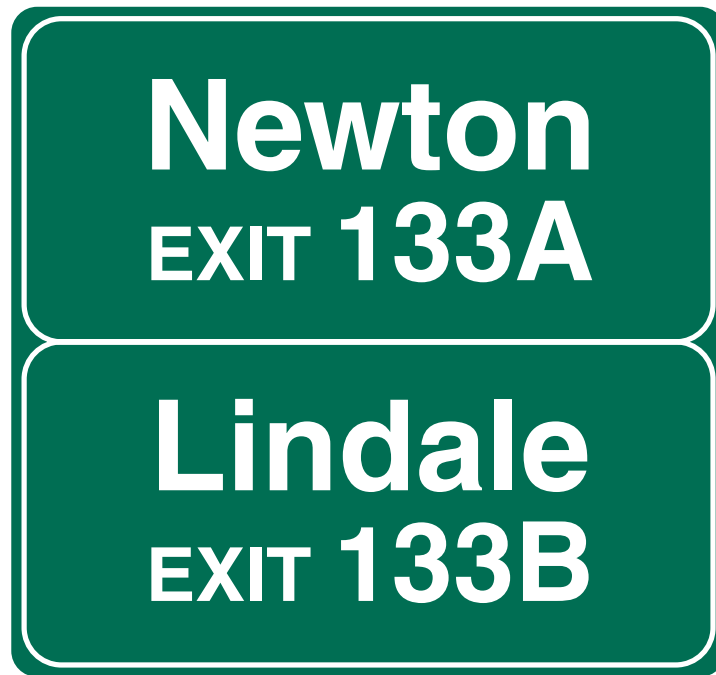
Figure 2E-17. Supplemental Guide Signs for Multiexit Interchanges
