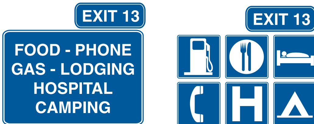
Figure 2E-41. Examples of General Service Signs (with Exit Numbering)
