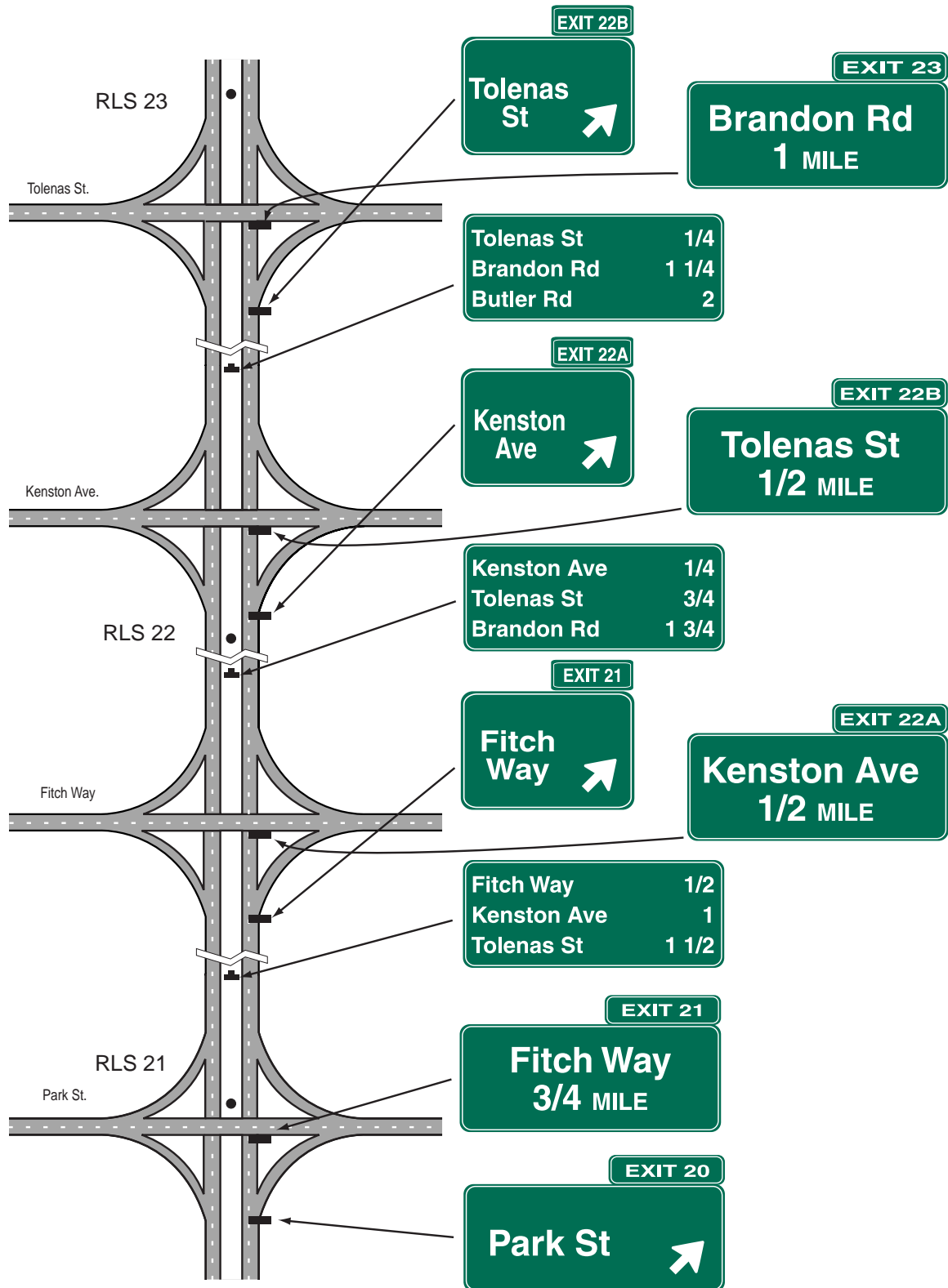
Figure 2E-23. Signing of Closely Spaced Interchanges Using Interchange Sequence Signs
