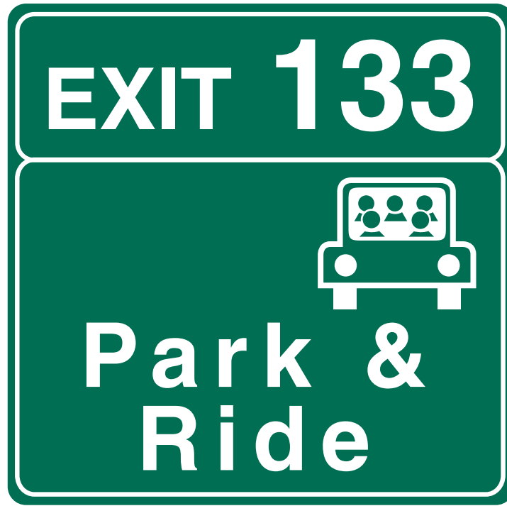
Figure 2E-19. Supplemental Guide Sign for a Park and Ride Facility (Route with Exit Numbering)
