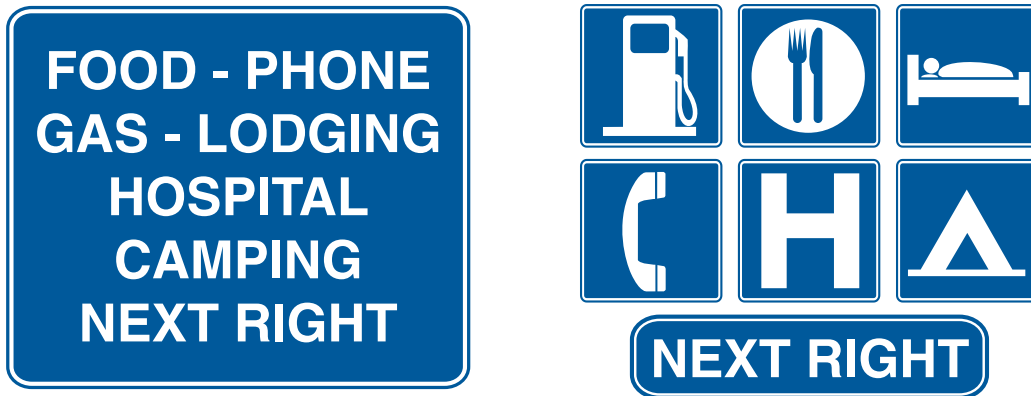
Figure 2E-40. Examples of General Service Signs (without Exit Numbering)
